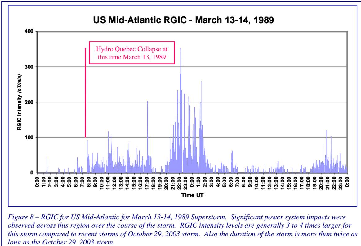
Figure 8 – RGIC for US Mid-Atlantic for March 13-14, 1989 Superstorm. Significant power system impacts were observed across this region over the course of the storm. RGIC intensity levels are generally 3 to 4 times larger for this storm compared to recent storms of October 29, 2003 storm. Also the duration of the storm is more than twice as long as the October 29, 2003 storm.
