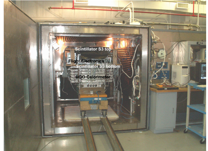
Fig. 4. The set-up for the temperature calibration in the thermal vacuum chamber at CSBF, Palestine, TX.
