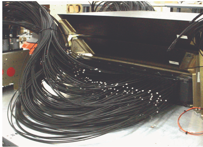
Figure 10. Calorimeter mounted under graphite targets during assembly of the calorimeter module. Shown in the foreground are the IFO fiber bundles carrying light signals through light-tight wall to a readout box.
