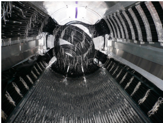
Fig. 8. Layout of MTOF with both-end readout using fiber-bundled light guide.
