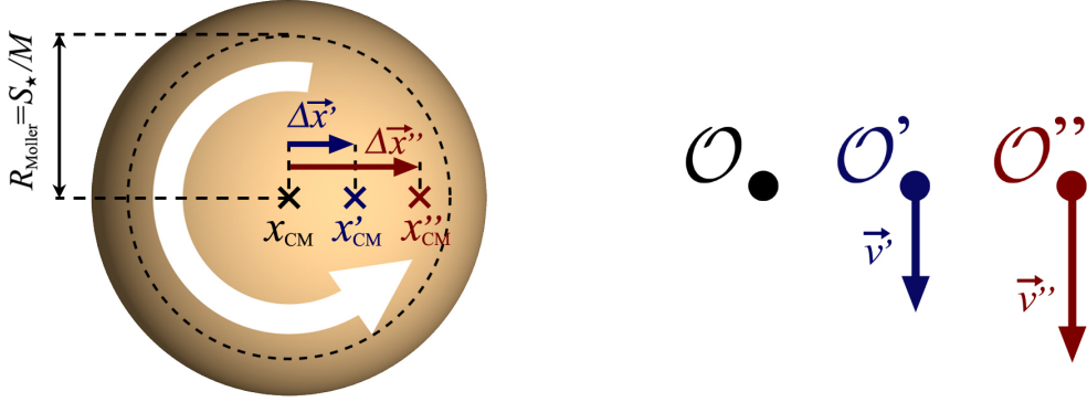
Figure 1: A free spinning spherical body in flat spacetime. Observer \mathcal{O} , at rest relative to the axis of rotation, measures the centroid x_{\text{CM}}^\alpha to coincide with the sphere's geometrical center (and with the rotation axis). x_{\text{CM}}^\alpha \equiv x_{\text{CM}}^\alpha(P) is the centroid as measured in the P^i = 0 frame. Observers \mathcal{O}' and \mathcal{O}'' moving (relative to \mathcal{O} ) with velocities \vec{v}' , \vec{v}'' opposite to the rotation of the body, see points on the right side of the body moving faster than those on the left side; hence for these observers the right side of the body is more massive, and the centroid they measure is shifted to the right by \Delta\vec{x} = \vec{v} \times \vec{S}_*/M . The larger the speed v the larger the shift; when v equals the speed of light, the shift takes its maximum value, with the centroid lying in the circle of radius R_{\text{Moller}} = S_*/M .
