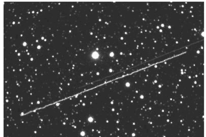
Fig. 13. Distant geosynchronous satellite passing the star HD52265 illustrates the 4-inch telescope’s sensitivity to orbiting objects (exposure = 95s, FOV 18' \times 26' ). Although these satellites are large, the strength of this trace suggests that smaller objects could be detected at this distance (35,786km). A satellite orbiting even farther away would be moving more slowly, possibly still detectable as its light would be spread over fewer pixels.
