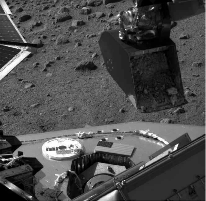
Figure Epilogue.1. NASA's Phoenix Mars Lander poised to deposit a soil sample into one of its ovens, where samples were heated to determine their chemical composition. (NASA)
