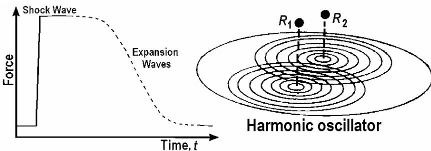
**Figure 10.4** a) General shape of a simple shock wave. b) If shocks oscillate harmonically they may undergo constructive and destructive interference.
