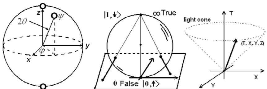
**Figure 11.20** The qubit. (a) Block Sphere representation of a qubit, a geometrical representation of the pure state space of a two-level quantum mechanical system. Alternately, it is the pure state space of a 1 qubit quantum register. (b) Stereographic projection model of a qubit on a complex Riemann sphere. (c) Relativistic model of a qubit with interacting quantum fields.
