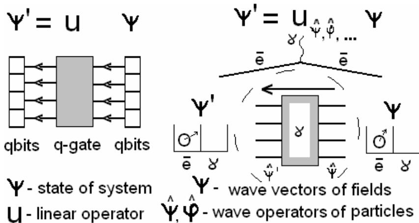
**Figure 11.21** (a) Usual q-gate with constant number of states and particles. (b) Relativistic quantum bit (r-qubit) with constant particles but variable or infinite states.
