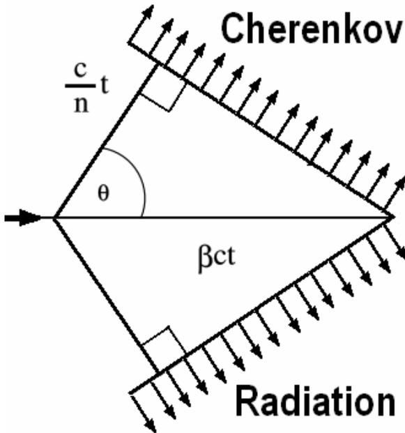
**Figure 10.3** Geometry of Čerenkov radiation. In the figure,  $v$  is the velocity of the particle (arrow),  $\beta$  is  $v/c$  and  $n$  is the refractive index of the medium. The arrows are the direction of Čerenkov radiation so that  $\cos \theta = 1/n\beta$ .
