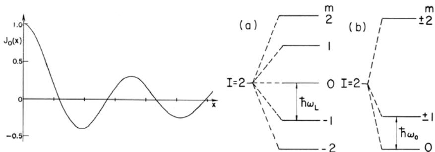
**Figure 11.19** (a) Graph of Bessel function  $J_0(x)$  showing how  $J_0$  oscillates as  $x$  increases. (b) Nuclear energy splitting of substates for total spin 2 in a magnetic field and (c) axially symmetric electric field with quadratic energy splitting,  $\omega$  is the spin precession frequency.
