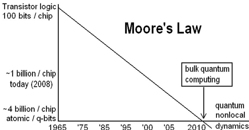
**Figure 11.2** Moore's law states that since the invention of the integrated circuit in 1958, the number of transistors on a chip doubles about every two years, as well as the processing speed, accompanied by a corresponding reciprocal shrinkage in the size of a transistor [1]. Right on schedule the Intel Itanium had 1 billion transistors in 2008. The graph predicts quantum computing should appear by the year 2011 unless a phase effect delay occurs from Schnell's Law.
