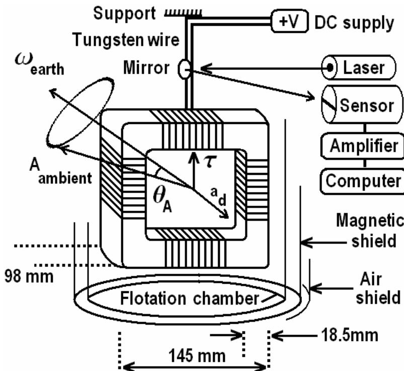
**Figure 7.8** An electric current in a toroid produces a dipole field which interacts with the ambient vector potential producing a torque on the toroid which varies with the Earth’s rotation. Fig. redrawn from [76].
