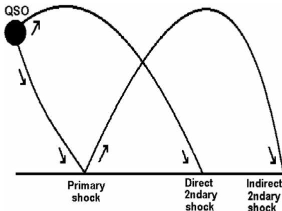
**Figure 10.6** A conceptualization of a direct and indirect secondary boom. Figure redrawn from [60].
