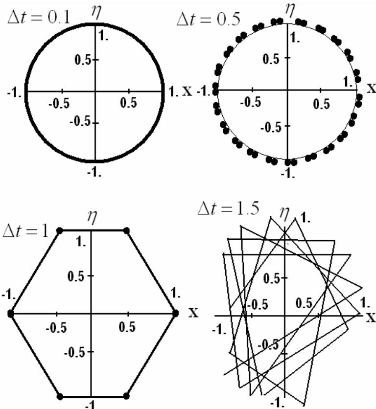
**Figure 11.22** Numerical simulation of phase space trajectory for Dubois' superposed incursive oscillator based on coordinates and velocities  $x_n = 1/2[x_n(1) + x_n(2)]$ ,  $v_n = 1/2[v_n(1) + v_n(2)]$  is shown for values of  $\Delta\tau = \omega t$  equal to 0.1, 0.5, 1.0 and 1.5. Initial conditions are  $\chi_0 = 1, \eta_0 = 0$  and  $\tau_0 = 0$  with total simulation time  $\tau = \omega t = 8\pi$ . Figure adapted from [6,68].
