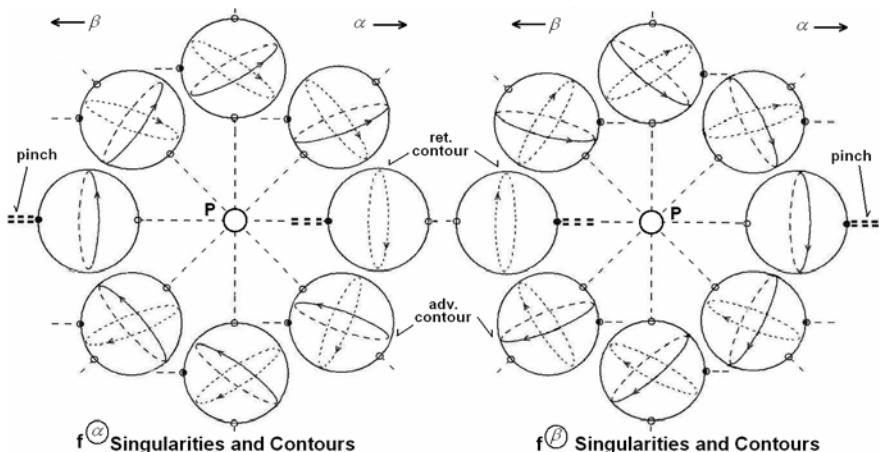
**Figure 11.28** Contours and singularities of two linearly independent advanced (solid lines) and retarded (dashed lines) fields that can be computed by contour integration.
