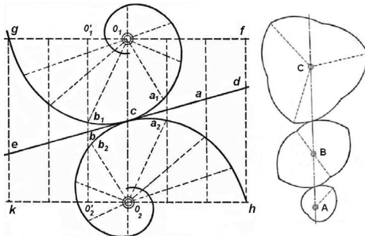
**Figure 12.6** Perfect rolling motion allows a resonance hierarchy to be set up at the points of contact that are in phase. Here logarithmic spirals are used to conceptually illustrate the hierarchical coupling concept.
