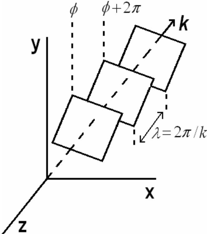
**Figure 5.17** Planes or surfaces of constant phase,  $\phi$  along the  $z$  axis for the plane wave propagation vector  $k$ .
