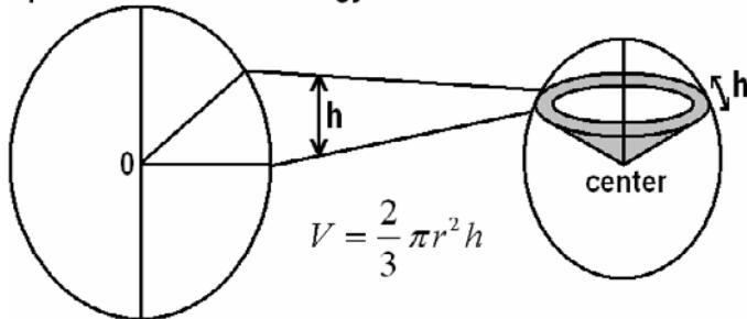
**Figure 5.18** Spherical sector, a volume formed by rotating a section of a circle around a diameter.
