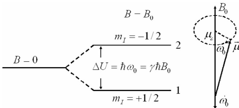
**Figure 9.14** a) The two magnetic energy states for the spin,  $I = 1/2$  single proton of a hydrogen atom in a magnetic field. b) Time variation of the magnetic moment of the proton in magnetic field  $B_0$  with precession frequency  $\omega_0 = \gamma B_0$ , the fundamental resonant frequency from a).
