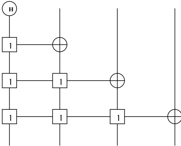
**Figure 11.32** Quantum Circuit for the GHZ state.
