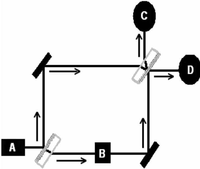
**Figure 9.1** General form of the Mach-Zehnder interferometer used to determine the phase shift caused by a sample placed in the path of one of two collimated laser beams. A is the beam source, B the sample and C & D the detectors. Note the two types of mirrors.
