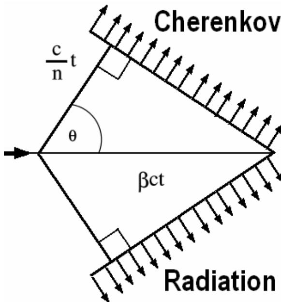
**Figure 10.3** Geometry of Cherenkov radiation. In the figure,  $v$  is the velocity of the particle (arrow),  $\beta$  is  $v/c$  and  $n$  is the refractive index of the medium. The arrows are the direction of Cherenkov radiation so that  $\cos \theta = 1/n\beta$ .
