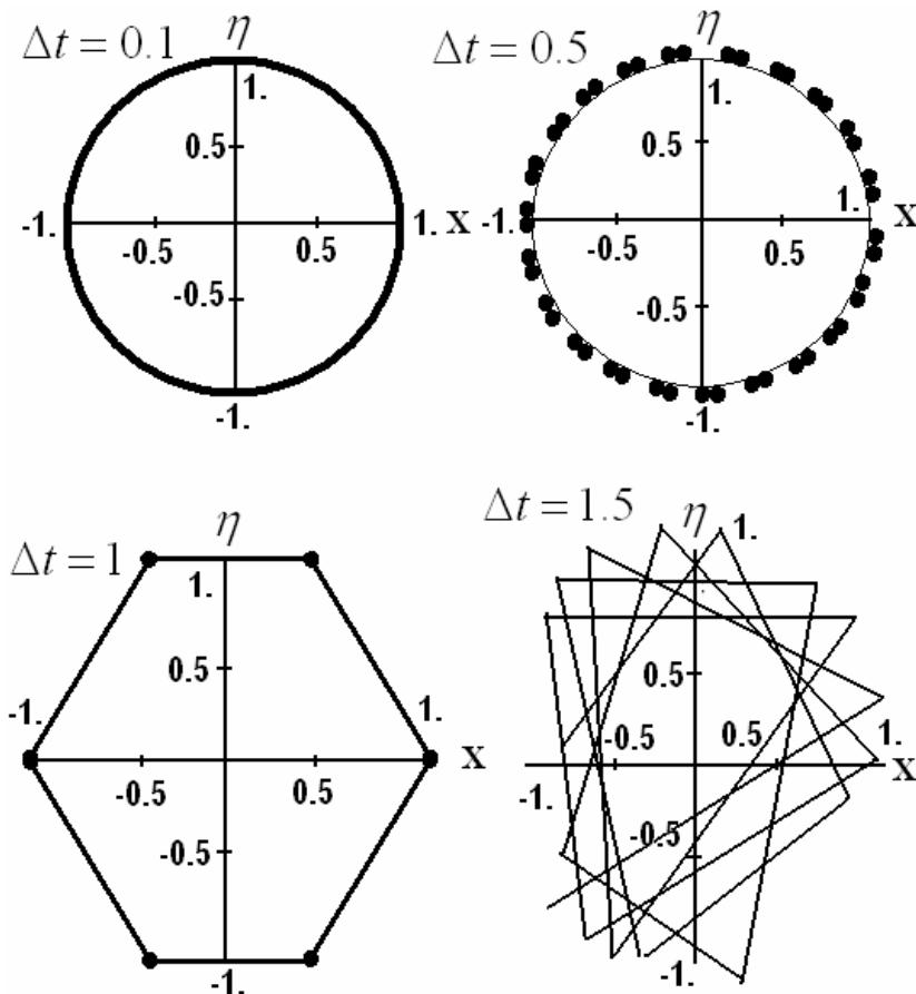
**Figure 9.13** Numerical simulation of the phase space trajectory of the Dubois superposed incursive oscillator based on coordinates and velocities  $x_n = 1/2[x_n(1) + x_n(2)]$   $v_n = 1/2[v_n(1) + v_n(2)]$  is shown in the figure for values of  $\Delta\tau = \omega t$  equal to 0.1, 0.5, 1.0 and 1.5. Initial conditions are  $\chi_0 = 1, \eta_0 = 0$  and  $\tau_0 = 0$  with total simulation time  $\tau = \omega t = 8\pi$ . Figure adapted from [82-85].
