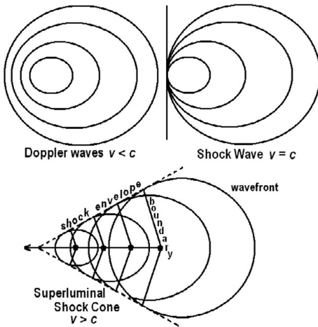
**Figure 10.2** Simplistically considering a shock as originating from a point source in two dimensions the disturbance forms circular wavefronts centered at successive positions of the QSO's harmonic gravitational image source as illustrated at the bottom of the Figure. The wavefronts overlap and form the shock envelope. In 2D the shock envelope is a wedge, and in 3D it forms a cone.
