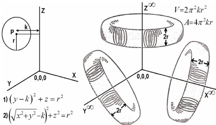
**Figure 5.19** a) Generator of a toroidal surface formed by rotating a circle, P of radius,  $r$  at distance,  $k$  from the rotation axis,  $z$  in the plane of the circle. b) Spherical sectors from Fig. 5.16 modeled to form tori on the  $x,y,z$  axes to represent regions of equal phase.
