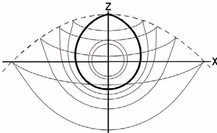
**Figure 10.7** Select wave-fronts, a caustic, locus of cusps, when  $Z = 1 - x^2 / 4$  plotted on the dashed line of a wave envelope. Figure adapted from [60].
