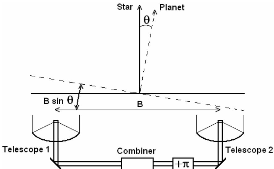
**Figure 13.1.** Two telescope space-based nulling interferometer, simplest configuration for producing a dark fringe in the line of sight when properly phased. This destructive interference enables planet detection by subtracting stellar coronas when focusing the null region on the stars disk. Redrawn from [63].
