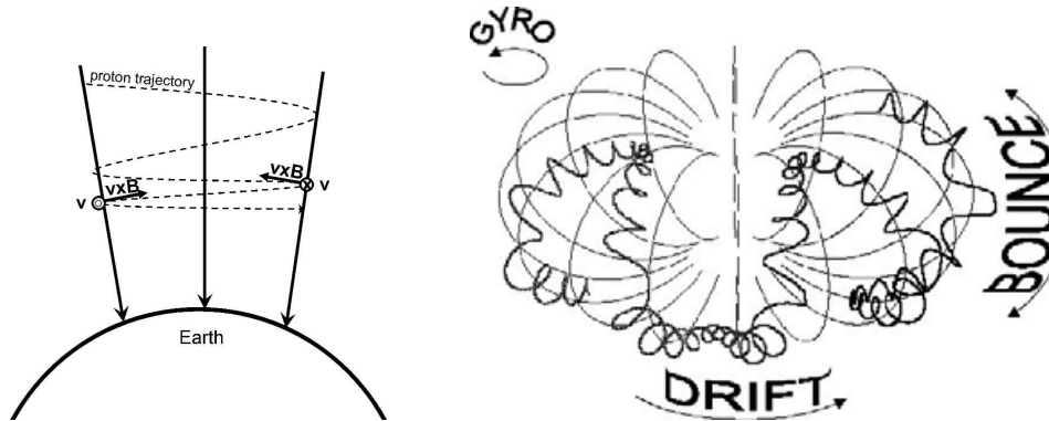
Fig. 8.1. (left) Schematic diagram showing the Lorentz force as a particle moves into the magnetic field gradient at Earth's poles. [Fig. H-II:11.2] (right) Schematic diagram of particle motion in a dipole magnetic field. [Fig. H-II:11.4]
